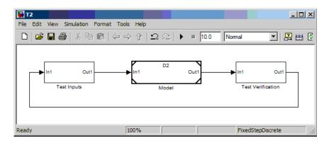
**2** Simulate the T2 model to run component C in PIL mode and test its RTW model reference target.
