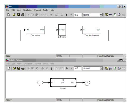
To create stand-alone code, perform a subsystem build of D\_Subsys. The stand-alone code calls the RTW model reference target of component C.
