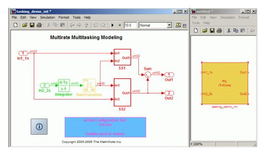
For a right-click subsystem build, you get a PIL block that represents the subsystem. You can test the deployable standalone object code, for example, by copying the PIL block into the original model to replace the original subsystem.
