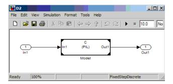
To create stand-alone code, perform a top-level build of D2. The stand-alone code calls the RTW model reference target of component C.
